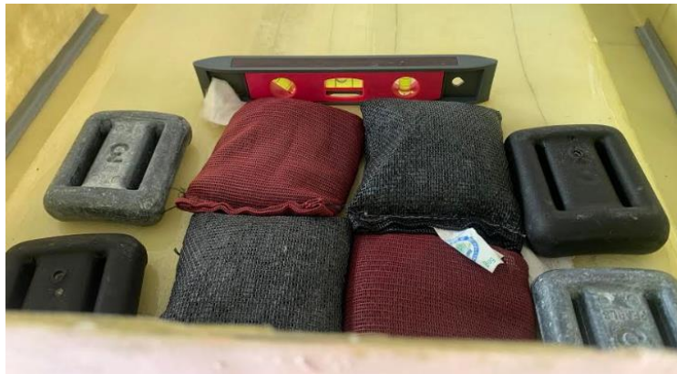
Image 27. The dive weights placed in the hull during the deflection test
