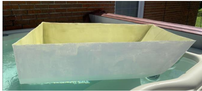
Image 23. The boat hull floating while carrying 24 pounds for 30 minutes with no leakage
