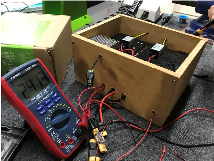
Measured voltage for one of the ESCs.
