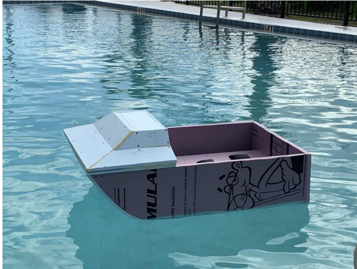
Image 9. The boat mold floating with 12 lbs. of weight applied
