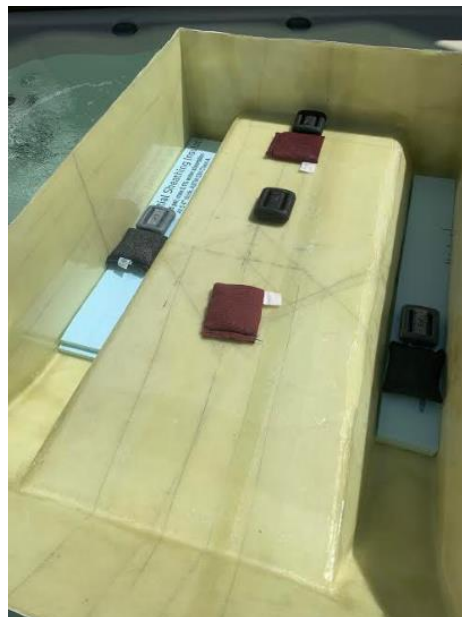
Image 24. The floatation test with the dive weights distributed correctly.
