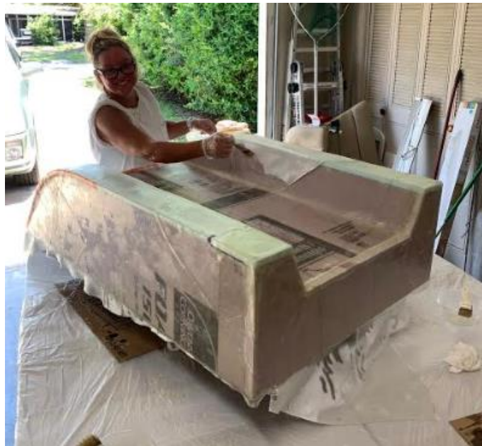
Image 10. Hand Lay-Up of Fiberglass
